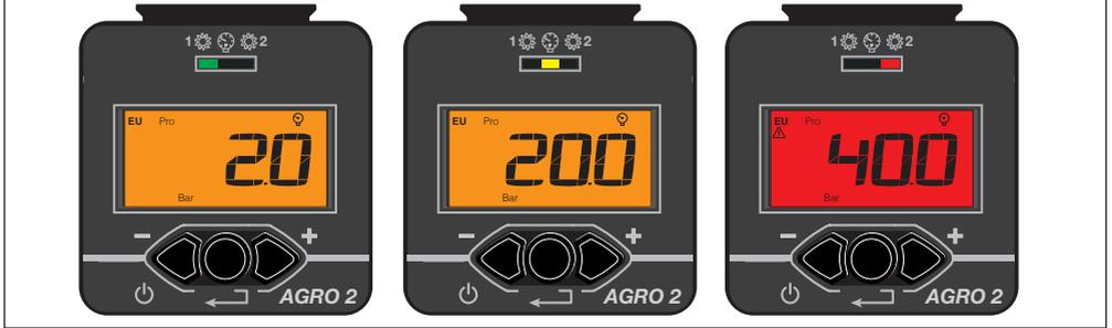
The full scale value of the transducer is chosen. The set values are: 10 - 16 - 25 - 60 - 100 - 250 - 400 - 600 - 1000 - 1500 BAR.
