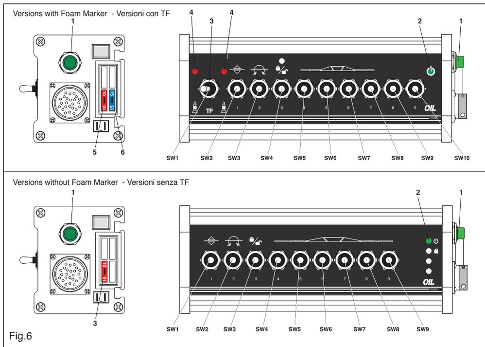
The box is switched on with the green button on the right side (pos. 1), the green LED on the front (pos. 2) signals the power. The momentary switches can control double-acting hydraulic valves. On the front are positioned:
