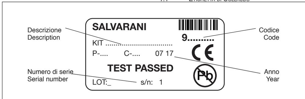
A test label is placed at the bottom of the box, where code and product description, year of production and serial number are indicated.
