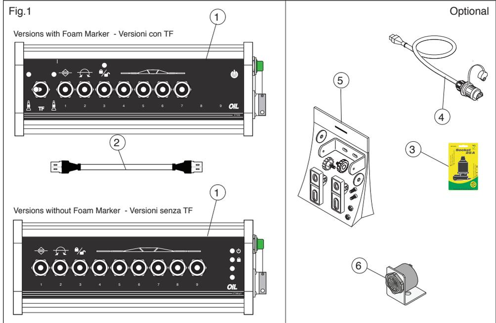
The wiring can be separated from the control box by means of a connector.
